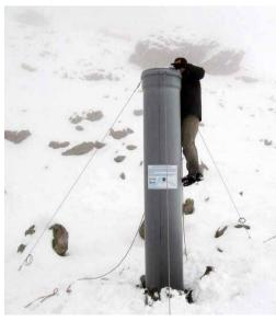
FIGURE 1: Maintenance of a cumulative precipitation gauge, Savoie, 2200m, photo University of Savoie, EDYTEM (FR)
